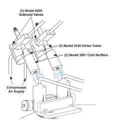
**The Problem:** Automobile fuel tanks are blow molded, then clamped to a fixture to prevent distortion during the cooling cycle. The cooling time of over 3 minutes required for each tank created a bottleneck in the production process.
