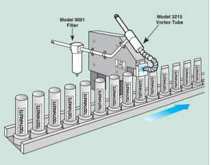
throughput. The vortex tube is the low cost solution for cooling parts, chambers, heat seals and various processes. They're easy to use, can be adjusted to produce cold air down to  $-50^{\circ}$ F ( $-46^{\circ}$ C) and have no moving parts to wear out.
